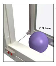
Possible Fall Hazard: Young children may fall out of the window if the window fall prevention device is not installed correctly. When properly engaged, no space shall exist at the lowest opening portion of the window opening that would permit the passage of a rigid sphere measuring 4" (102) in diameter.
