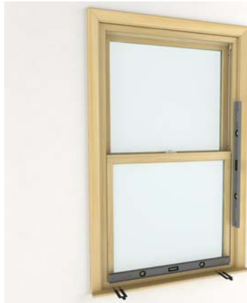
Figure 3 Center, shim, and fasten the unit in the opening.
